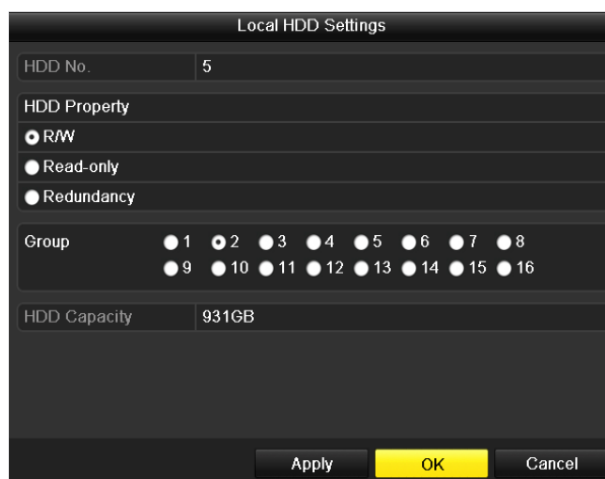
Figure 10. 15 Local HDD Settings Interface
