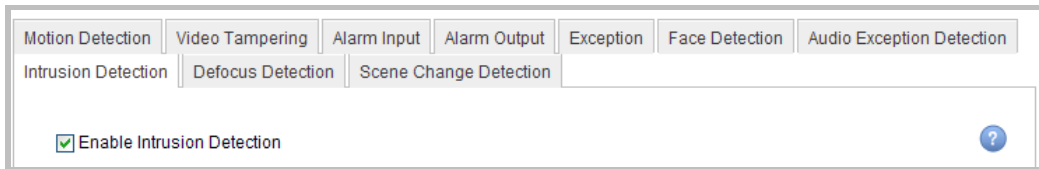
Figure 6. 11 Setting Intrusion Detection on IP Camera
