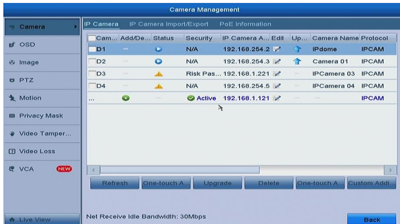
Figure 2. 19 Adding IP Camera Interface
