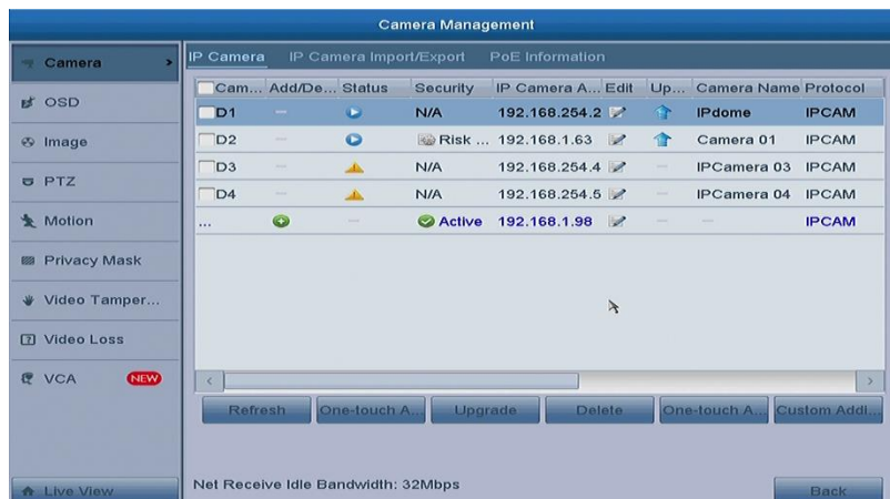
Figure 2. 15 IP Camera Management Interface
